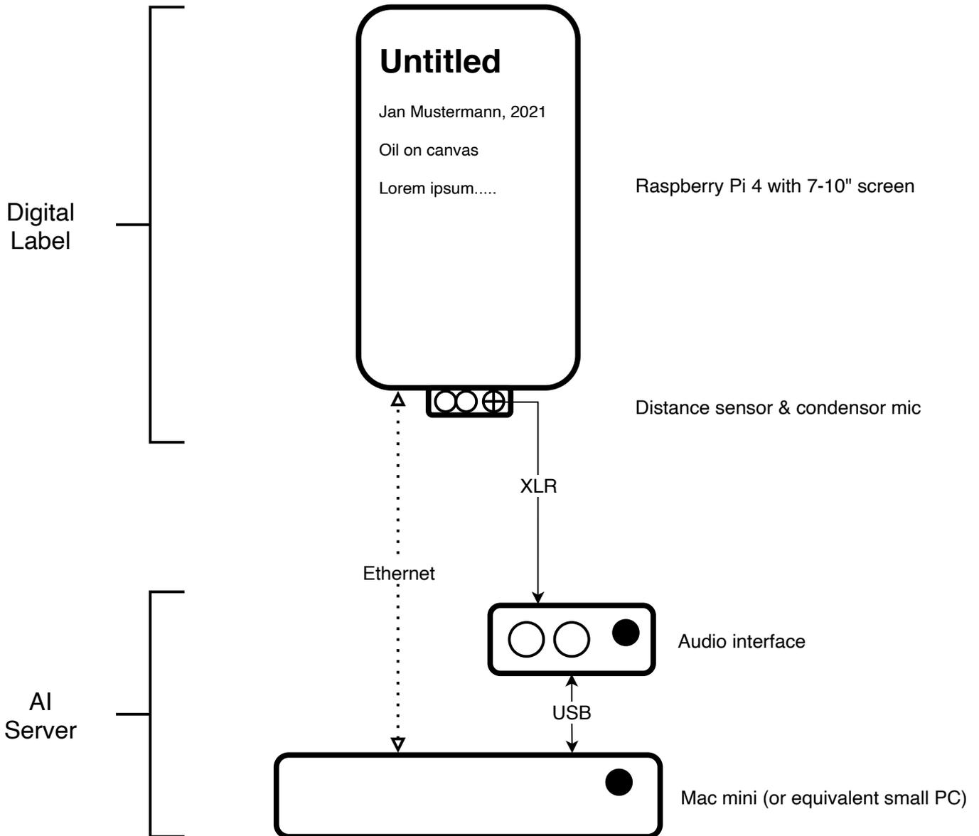
Digital label is mounted on wall for presentation. AI Server and audio interface are to be hidden.
